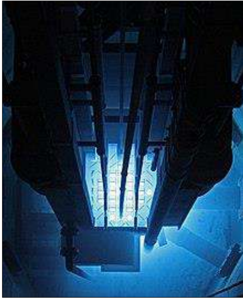
Fig 1.1: Cherenkov radiation in the University of Massachusetts Lowell Radiation Laboratory [60]
